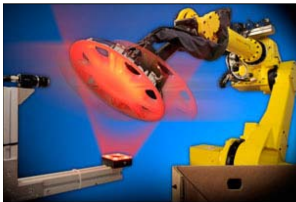
A FANUC robot presents a hub cap to a vision system for quality inspection before loading it into machine for assembly.
