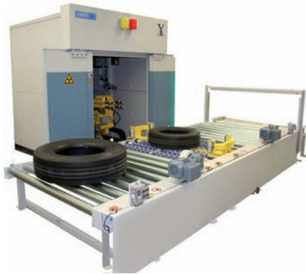
Above: The Yxlon TireAxis software automates the Y.MTIS modular inspection system (above right)
